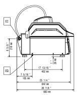
Electrical inlet (power) EO Electrical Outlet
